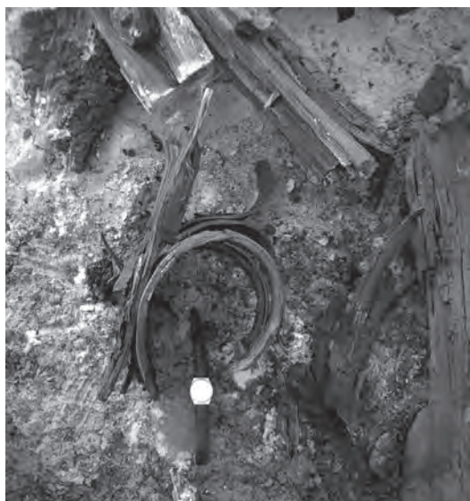
Fig. 6 Fragments of sapwood that curled rapidly when exposed to sunshine, suggesting low cellulose content.
